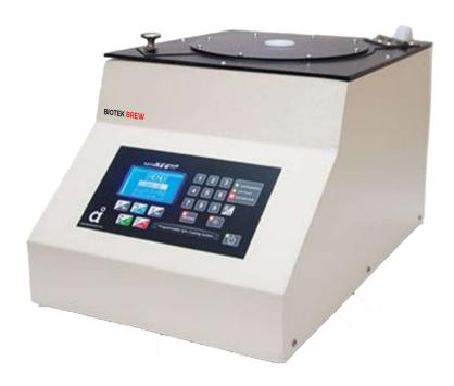
Spin Coating is a process in which solution is spread evenly over a surface using centripetal force. Spin coating will result in a relatively uniform thin film of a specific thickness.
